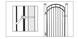
5. First, attach the catch (C) to the latch finger (C) while the gate (A) is in the closed position to ensure proper alignment. Then, position the catch (C) against the post where it naturally sits.
