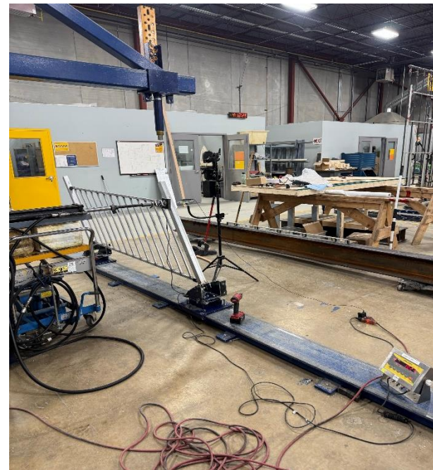
Photo No. 6 Horizontal Concentrated Load Test at Top of Post.
